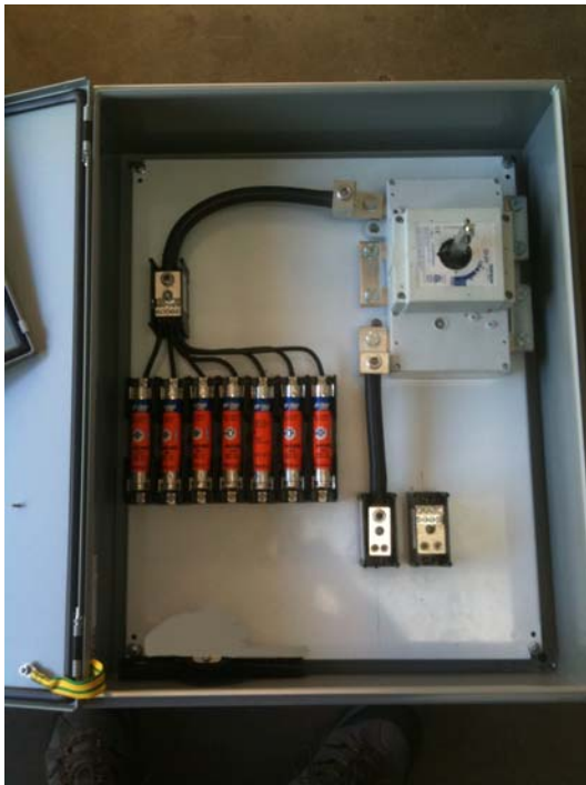
7 Input Re- Combiner With Disconnect Shown
